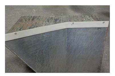
5. Remove the white plastic covering from the foam tape applied to the pods in step 2 and from the angle tabs applied in step 3.
