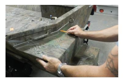
7. Use a  $\frac{1}{4}$ " drill bit to drill the 3 holes on each side at the same angle as the transom.
