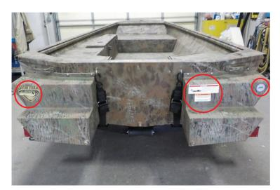
15. Inform the customer that the trailer tie down straps should now attach to the added pods. Additionally, let the customer know that the added buoyancy pods are not designed to support the weight of people, but can be used as boarding steps for dogs.
