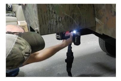
13. Now tighten the 3 bolts at the top of each pod. Extra bolt length can be cut off after tightening the bolt/nut.
