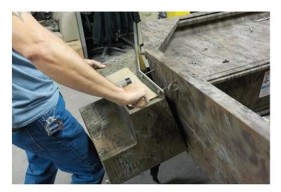
10. Install the washers and nuts on the bolts. Do not tighten at this time.
