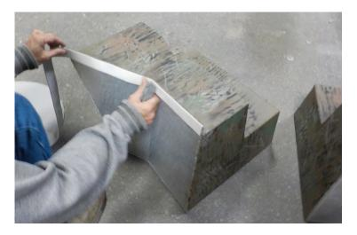
3. Drill 3 holes in the angle tab on each side of the transom using a #11 drill bit as shown. Remove the white protective covering from the adhesive side of the tape supplied in the kit and apply it to the angle tabs.
