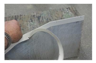
6. Hold the pod in place on the transom and mark the holes from the pod onto the transom. Mark the holes on both the starboard and port sides.
