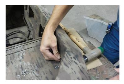
11. Push down on top of the pod while pre-drilling the three holes in the bottom of the pod through the angle tabs on the transom using a #29 bit.
