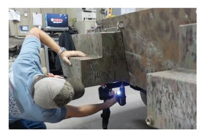
12. Install the 3 black screws in the bottom of each pod.
