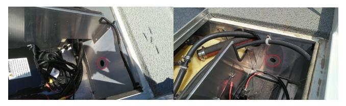
3. Inspect the foam in the holes to see it is visible within 0.25" of the wall.
