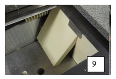
10. Install the sloped foam piece to the hull side.
