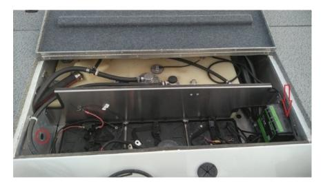
2. Remove black plugs in foam fill holes from both port and starboard sides.
