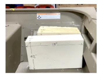
5. Place the pre-assembled starboard pod into place over the foam piece.
