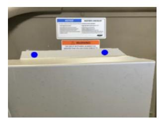
14. Drill two 7/16" holes (blue dots below represent drill location).
