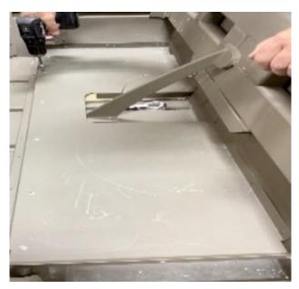
2. Lift up the gas pan and slide the two pieces of 15" x 5-1/2" x 1-1/2" foam (P/N: 895373) on the starboard side under the gas tank/battery pan.
