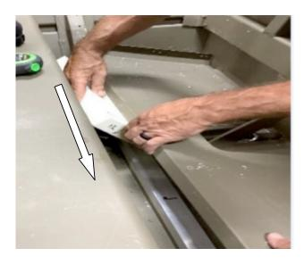
3. Put the gastank/battery pan back into place and secure it with AS66SS olive pop rivets (P/N: 73660266) using a pop rivet gun.
