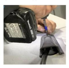
c) Visually insect the foam for gaps or visible spaces between the foam and the hull. If the gap or visible space is 1/2" or more, additional foam pieces must be installed in the boat per these instructions. Place tape around the cable cover area for better cleanup. Fill the space using Versi-Foam Kit (#73480035) into the cable cover areas. Read all the instructions on the Versi-Foam box before starting and follow them carefully.
