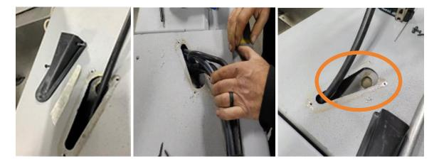
d) Re-install the cable covers set back into place and screw in the (3) black screws on the cable cover port and starboard side.
