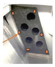
12) Next, install the aft bulkhead. First, remove the fire extinguisher bracket. Unscrew the (2) black screws and then set aside. Discard the black screws.
