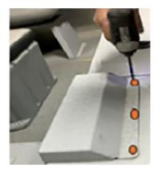
c. Install the (6) screws into the steering mount.
