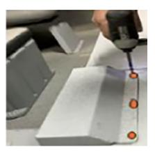
b. Unscrew the (6) black screws from the steering mount.
