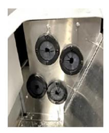
c. Secure the port rod holder in place with (7) #66 pop rivets.
