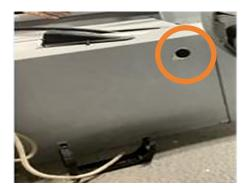
d) Tape the plastic around the area that will be inserted with foam for better cleanup. Fill the space using the Versi-Foam Kit (#73480035) into the accessible area of the cable cover. Read all the Versi-Foam Kit box instructions before starting and follow them carefully.
